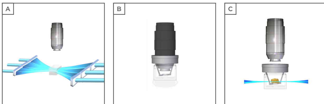
Figure 1: A schematic description of a commonly used ultramicroscopy-setup showing the bidirectional laser excitation of the sample.
