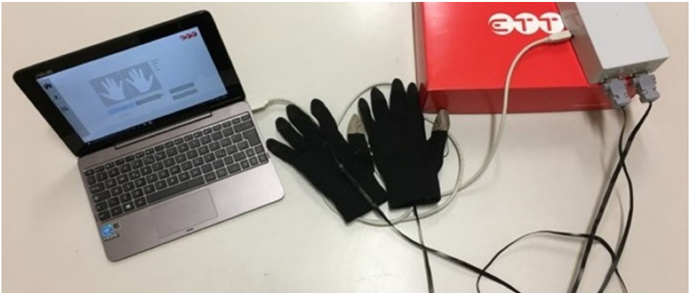
Figure 1: Hand Test System: an engineered glove that can be used to assess hand dexterity.
